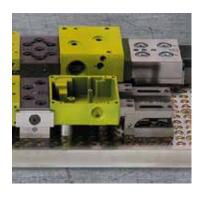
SPREITZER's modular fixturing and clamping systems provide innovative and powerful solutions for single-part and small series production. We manufacture compact and robust centre-clamping vises for their use on modern multi- axis machining centers.
