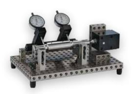
Concentricity gages from SPREITZER are used for test tasks on external, internal and flat surfaces of rotation parts. In particular, the concentricity of two or more diameters can be determined, and run-out measurements can be implemented.
